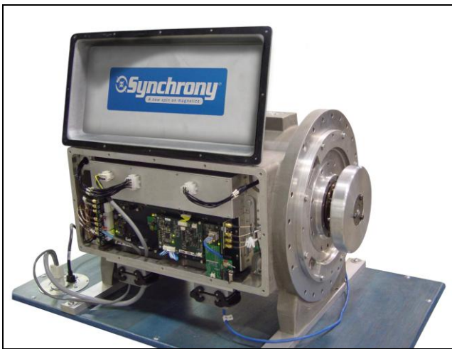
Figure 2: High speed drive train on magnetic bearings. Motor shown is 400-kW, 20,000-rpm.
