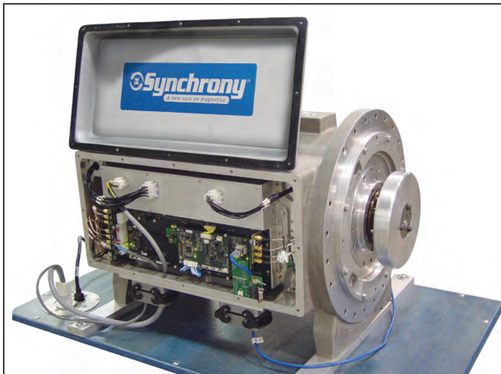
High-speed drive train on magnetic bearings. Motor shown is 400 kW at 20 000 r/min.
